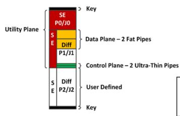
Figure 5-2 – HOST Payload Slot Profile, SLT3-PAY-2F2U-HOST
