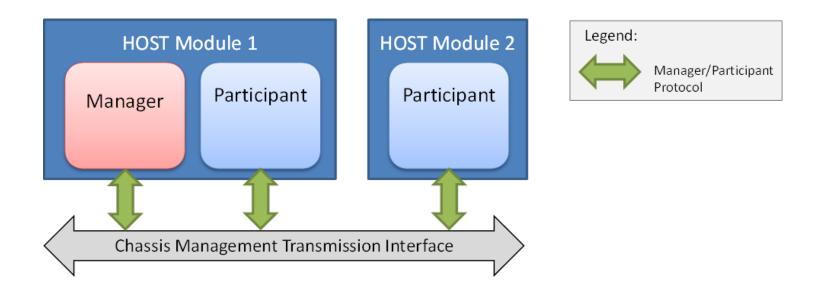
Autonomous subsystem that provides application independent hardware management and monitoring capabilities
